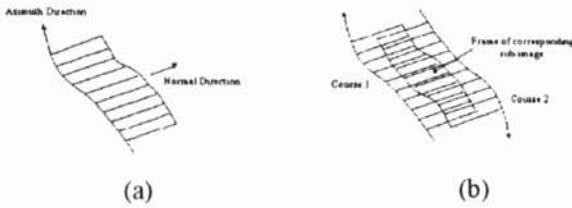
**Fig. 4. Frame determination of corresponding sub-images:** (a) Register to a global 2-D map; (b) Frame of corresponding sub-images.
