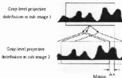
**Fig. 5. Motion estimation using gray-level projective distribution**
