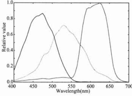
Figure 1. Spectral sensitivity functions of the camera.
