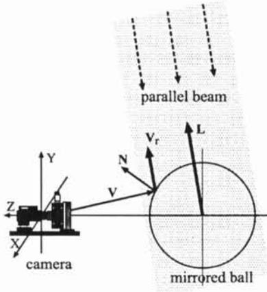
Figure 2. Geometric model of the observation.
