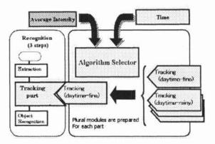
Figure 4: Dynamic Algorithm Selection in Moving Object Recognition Part
