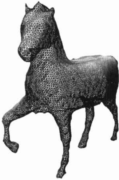
Figure 7: Triangulated mesh of the 3D model built from the silhouettes and the estimated motion.
