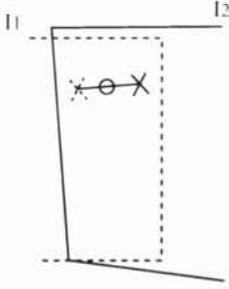
Figure 5: Feature correspondence for planar projective transform using three images
