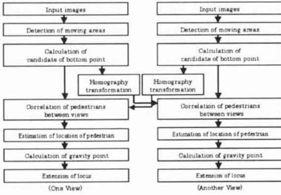
Fig.3: Flow diagram of proposal method
