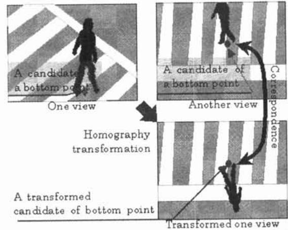
Fig.6: Homography transformation of a candidate of a bottom point
