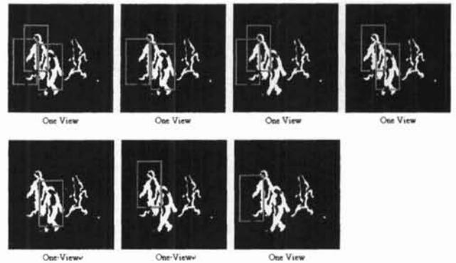
Fig.11: Combination of the rectangle to estimate the location of a pedestrian
