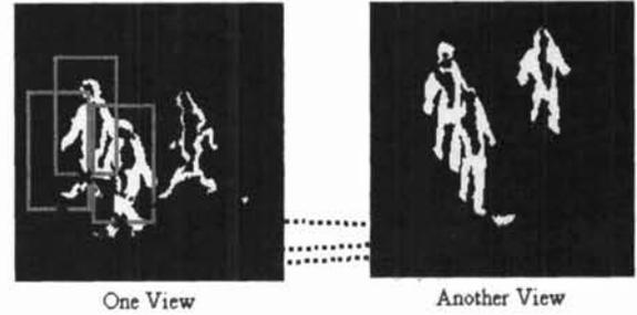
Fig.10: Setting of the rectangle to estimate the location of a pedestrian
