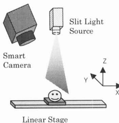
Fig.4 Experimental setup for 3D measurement
