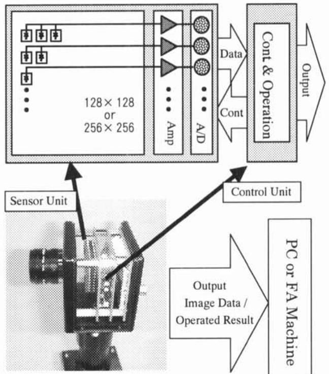
Fig.1 System structure
