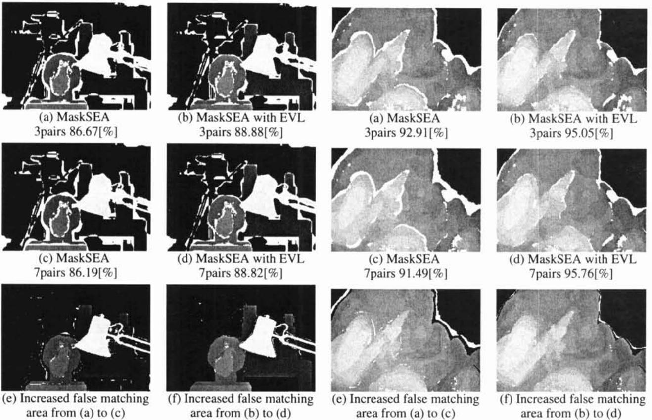
Figure 5: Robustness for mask pattern inconsistency. (a) (c) results by MaskSEA, (b)(d) results by proposed method. (a) and (b) are obtained by masks with 3 stereo pairs, (c) and (d) are obtained by masks with 7 stereo pairs. (e) and (f) indicate the increased false matching. Increase in (f) is less than that in (e).
