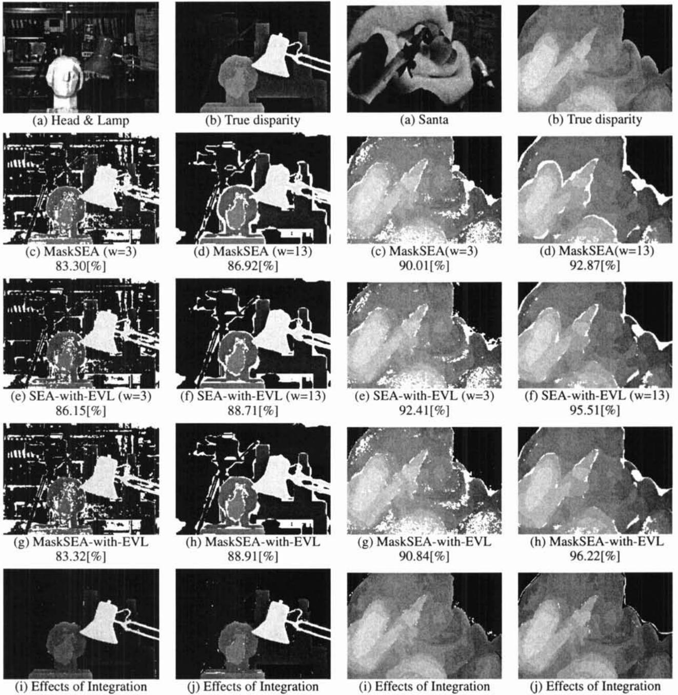
Figure 4: Effectiveness for large window size. (a) base image, (b) true disparity, (c) (d) results by MaskSEA, (e) (f) results by SEA-with-EVL, (g) (h) results by proposed method. In (c) to (h), false matching is shown by white. In (i) and (j), pixels where correct disparities were obtained only by the proposed method are indicated by white.
