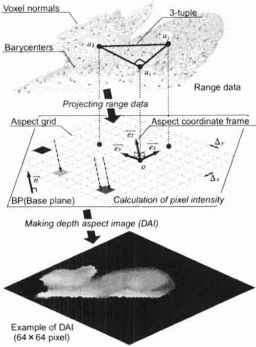
Figure 3: Procedure of making DAI.
