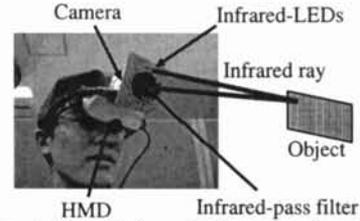
Figure 1: Active-infrared Camera for the WVT.
