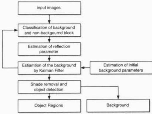
Figure 1: System flow of extraction process
