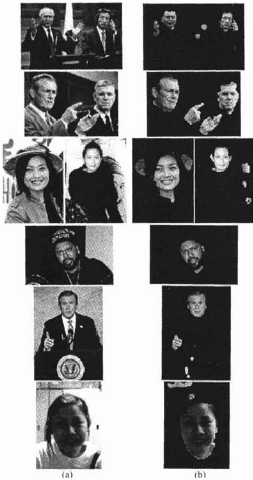
Figure 6: Skin-color extraction for face detection: (a) original image, (b) skin-color extraction result.
