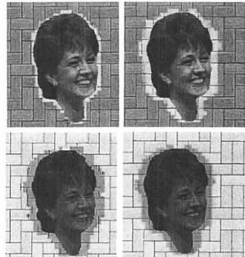
Figure 3: Top row: Stationary FG and moving BG for left Tritemporal and right reference ME (with \alpha_E = 0.5 always). Bottom row: both MEs for moving FG and stationary BG. Note that for a stationary FG object the tritemporal ME gives a negligible vector field mismatch, but for a moving FG it performs worse.
