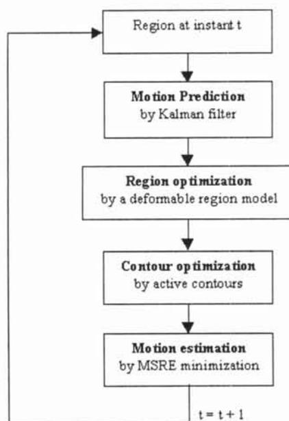
Figure 1: Tracking algorithm.
