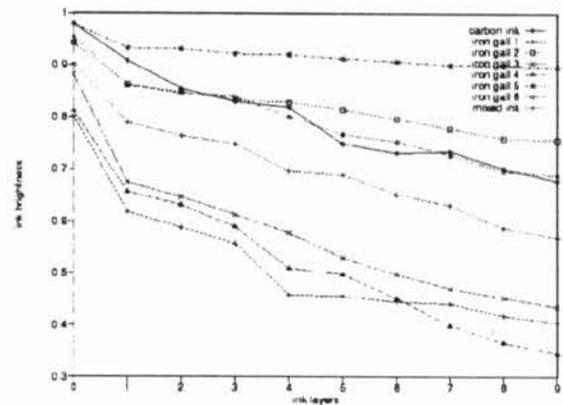
**Figure 5.** The intensity values of each ink under different thickness values form characteristic reflectivity lines.
