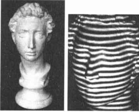
Figure 3: Sample target object (left) and projected fringe pattern (right).
