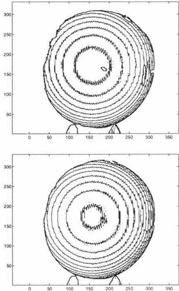
Figure 2: *Top*: Equal height contours representing the reconstruction of the ball using 5 color projection patterns. *Bottom*: Equal height contours representing the reconstruction of the ball using 10 black & white Gray code projection patterns.
