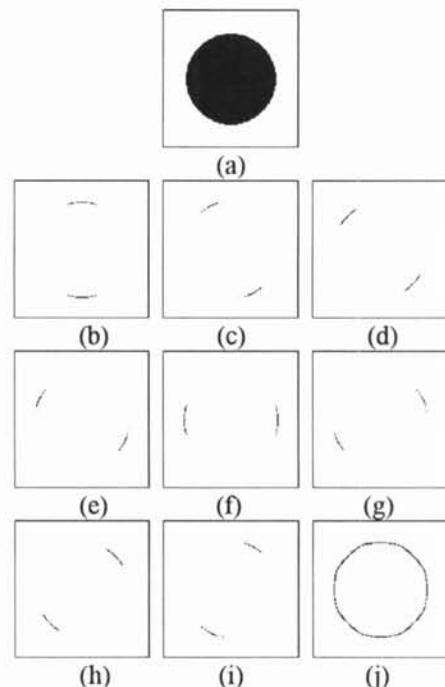
Fig. 5. Results of the orientation selective neural network for the image of circle ( $n=12, k=2$ ): (a) A circle image, (b)  $0^\circ$ , (c)  $26.6^\circ$ , (d)  $45^\circ$ , (e)  $63.5^\circ$ , (f)  $90^\circ$ , (g)  $116.5^\circ$ , (h)  $135^\circ$ , (i)  $153.4^\circ$ , and (j) the combined edges of (b)-(i).
