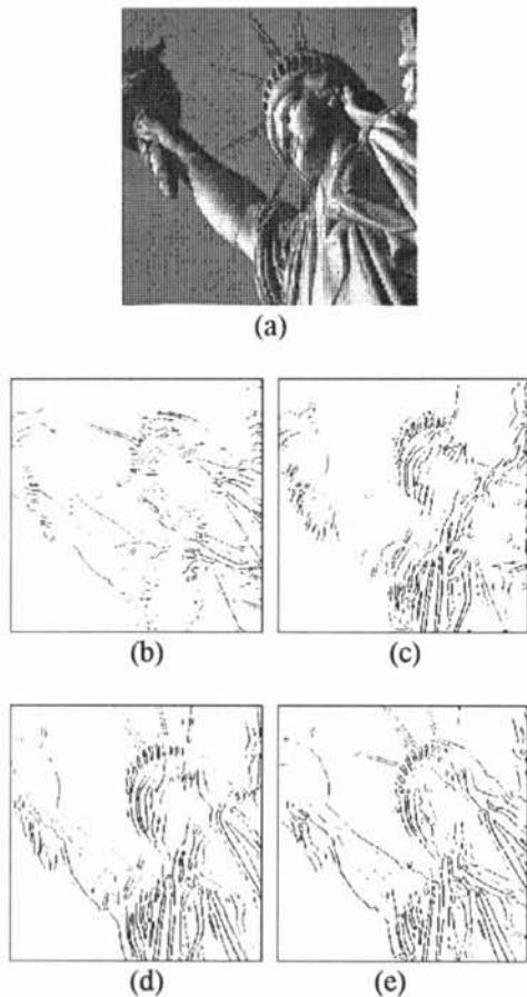
Fig. 6. The edges detected by the orientation selective neural network for Statue image ( $n=12$ ,  $k=2$ ): (a) Original image, (b)  $0^\circ$ , (c)  $45^\circ$ , (d)  $90^\circ$ , and (e)  $135^\circ$ .
