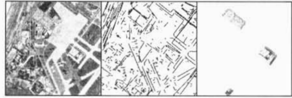
Figure 8: Left: A DD5 image over Berlin airport. Middle: Lines. Right: Building hypotheses
