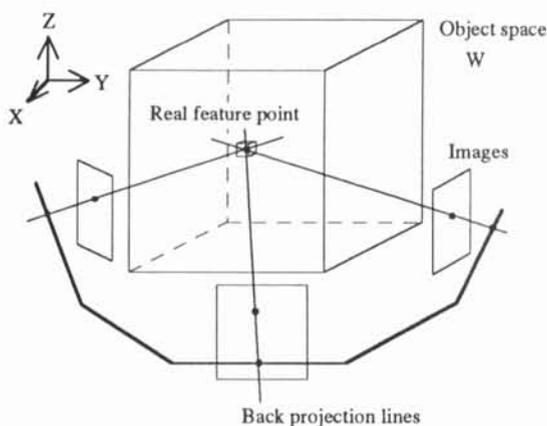
Fig. 1. The simple voting with back projection lines.
