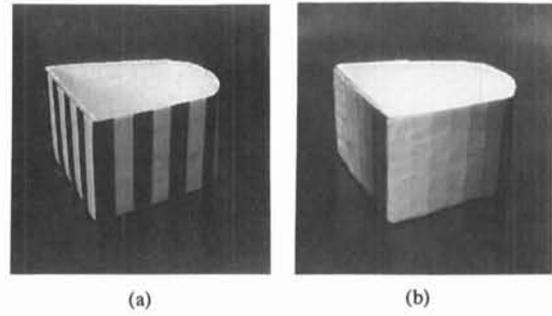
Fig. 3. The experimental object whose surface (a) has an obvious gray level, (b) has small variation of the gray level.
