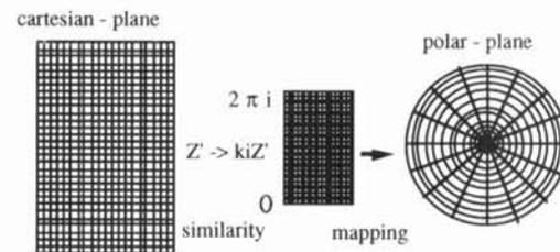
Figure 3 Mapping for the polar plane from the cartesian plane.
