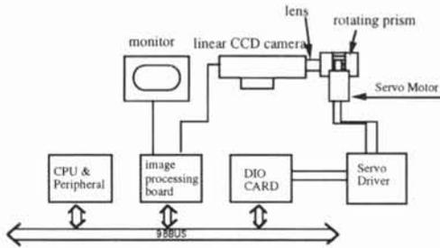
Fig. 8 System configuration to acquire the rotation image for retina-like sensor
