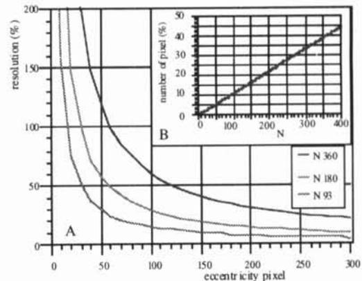
Fig6. (A). Percent variation of resolution as a function of eccentricity for different values of image line N. (B) Percentage of the number of elementer a given field as a function of N.
