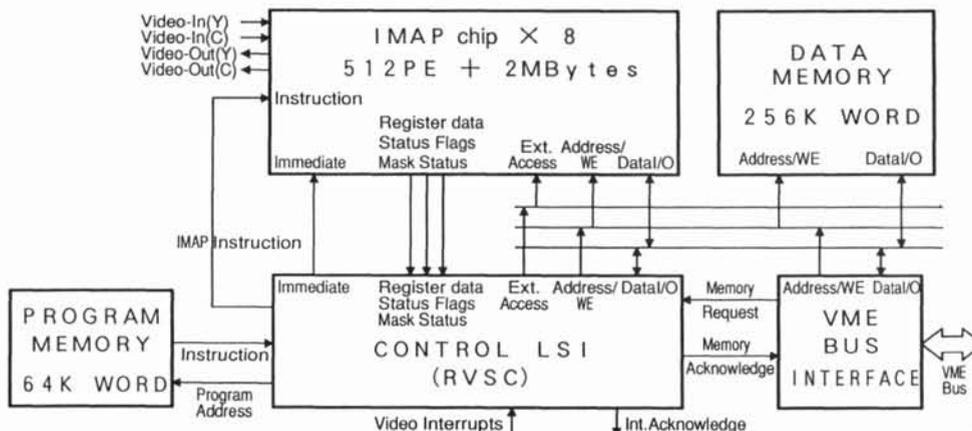
Figure 5 IMAP Board Configuration
