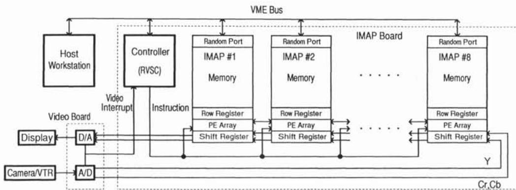
Figure 4 RVS-2 Configuration
