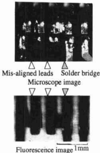
Fig. 13 Example of detected fluorescence image
