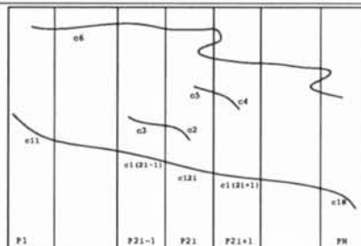
Figure 6: Various broken chains.
