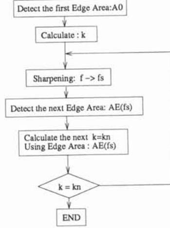
Figure 5: Processing flow for the adaptive image sharpening
