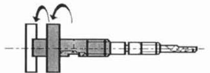
If there are still unrecognized blocks, the process is continued with a new starting point, if any is found. Here we start with the threading; the shaft is completely recognized to the left but propagation is stopped by a closing trapezoid to the right:
