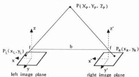
Fig. 2 The lateral stereo camera model.
