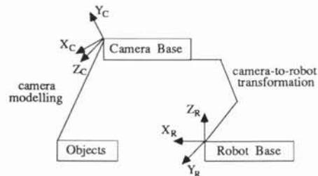
Fig. 1 Geometric relations in robot work space.
