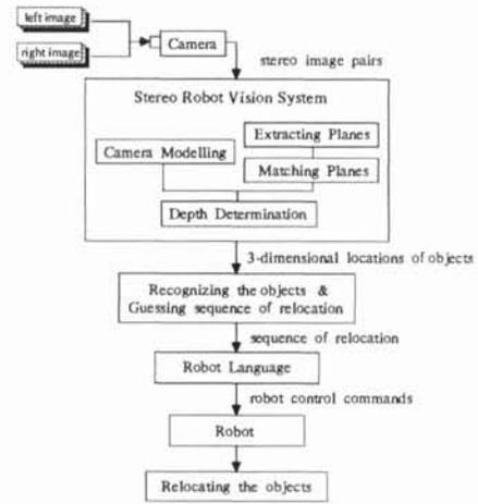
Fig. 3 The knowledge-based robot system implemented in this paper.
