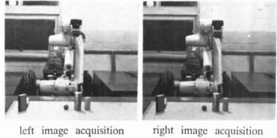
Fig. 4 Eye-on-hand camera configuration and stereo image acquisition from the lateral movement.
