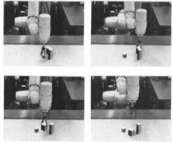
Fig. 8 The robot relocating objects in the order of height with minimum movements.
