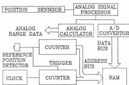
Fig.3 Block diagram of signal processing part.
