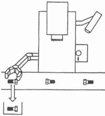
Fig.1 Vision system for parts feeder
