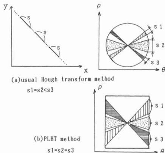
Fig.8 Geometric properties of the PLH function
