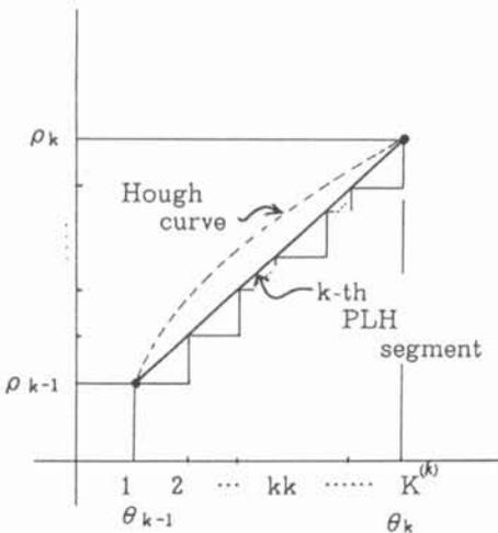
Fig.2 Incremental generation of PLH function
