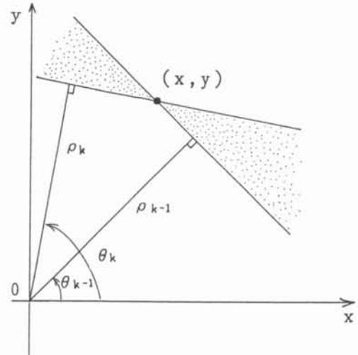
Fig.3 The behavior of the detected lines corresponding to a PLH segment
