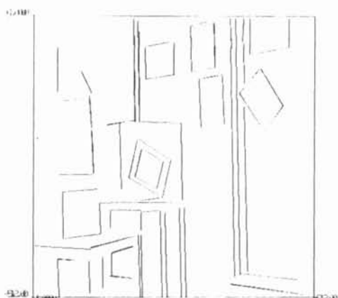
Figure 8: Reprojection on frame 2 of the reconstructed scene using the final computed motion (2 iterations) on all the segments of the scene.
