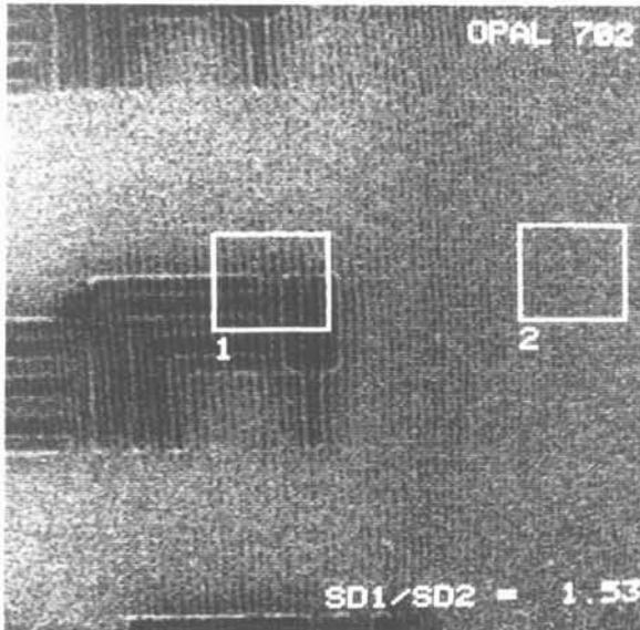
Figure 3: This SEM image was produced using probe current of 31 pA and 4 seconds collection time. The window size was 60x60 pixels.
