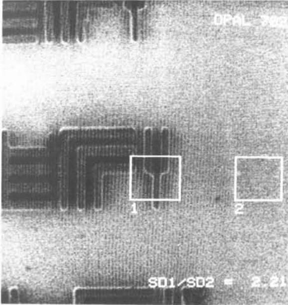
Figure 2: This SEM image was produced using probe current of 9 pA and 4 seconds collection time. The window size was 30x30 pixels, but was placed in different place (zone 2) on the image.
