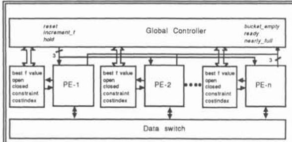
Figure 3. The architecture of the Path Finding Machine.
