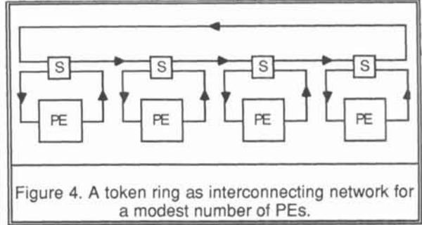
Figure 4. A token ring as interconnecting network for a modest number of PEs.
