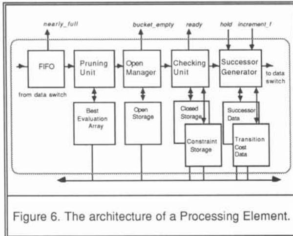
Figure 6. The architecture of a Processing Element.
