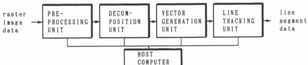
Fig.1 System block diagram.
