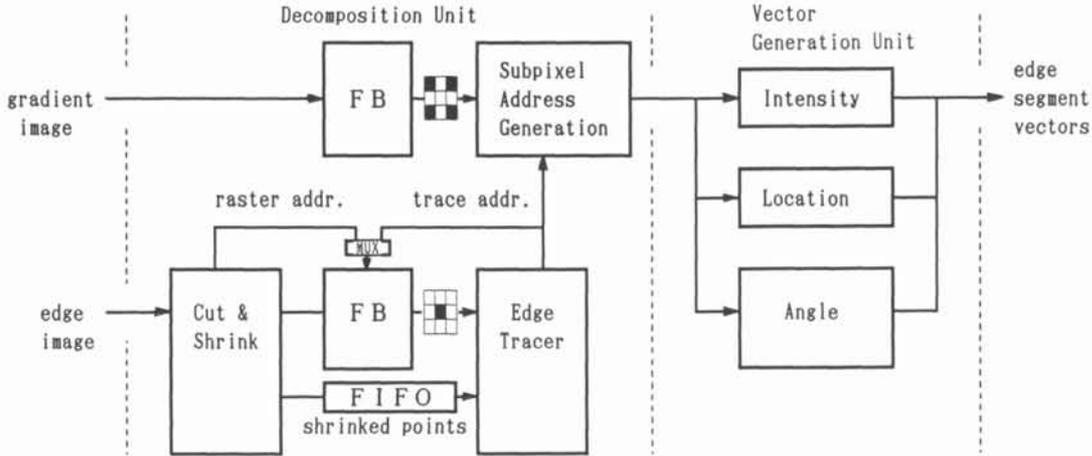
Fig.2 Decomposition Unit and Vector Generation Unit.
