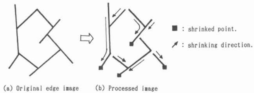
Fig.3 Overview of the Cut &amp; Shrink algorithm.
