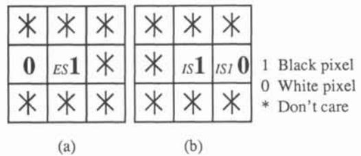
Fig.2 Necessary conditions for external start point(ES) and internal start point(IS)
