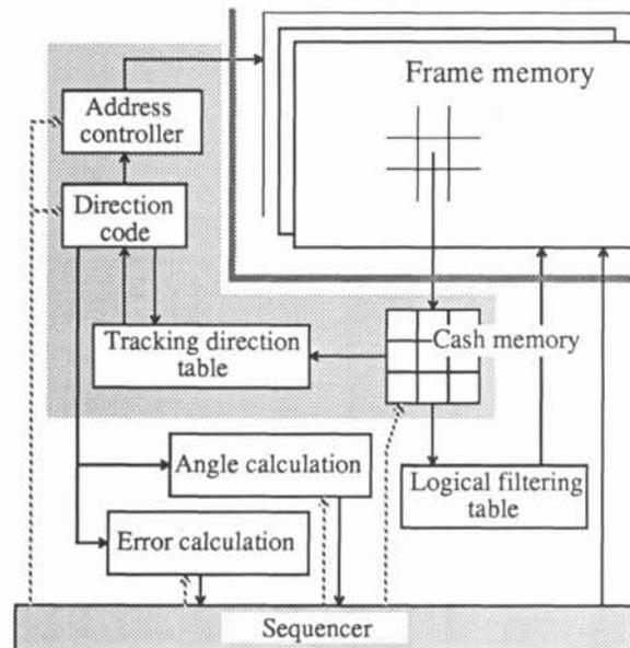
Fig.5 Configuration of contour tracking unit
