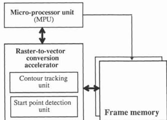
Fig.3 Block diagram of fast raster-to-vector conversion system
