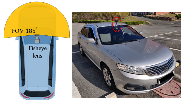
Figure 1. Fisheye lens camera installed on a front window of a test car
