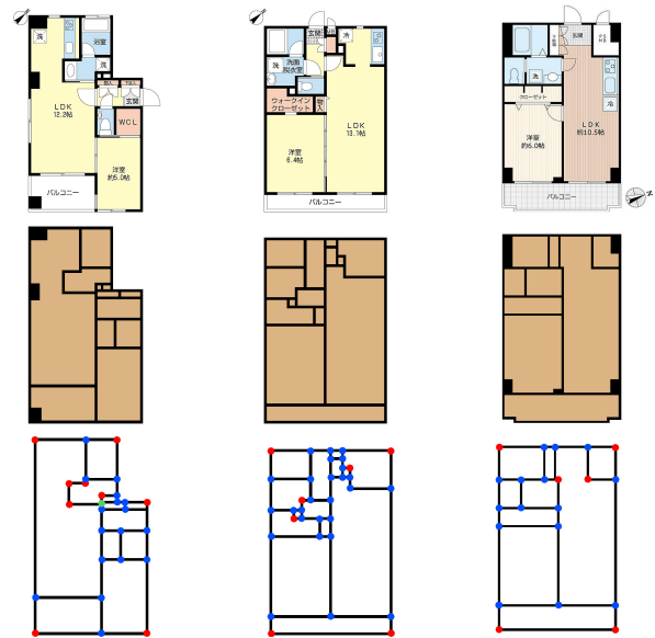
Figure 1: Floor plan matching. We define a distance between floor plan images based on the room layout. Instead of working with the input (top) or segmented images (middle), we use a graph representation (bottom), where edges represent walls and nodes represent intersections. Nodes are colored by degree.
