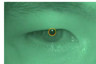
Figure 5. Result of pupil localization using anchor ellipse regression (in yellow) and mask segmentation (in red) under partial eyelid occlusion.
