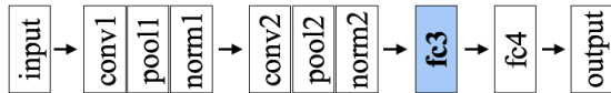
Figure 4. CNN structure for the experiments. This architecture is used for extracting CNN features and classifying frames of a gait sequence.
