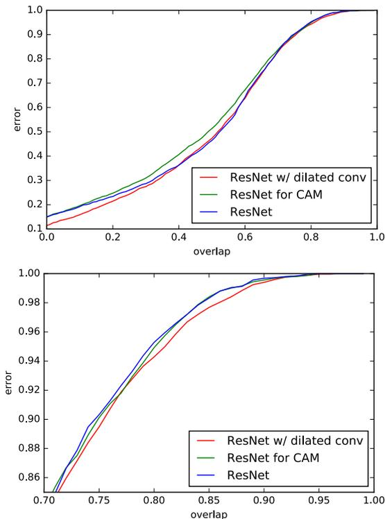
Figure 4. Localization error curves of the CNNs for overlap  $x$ . The top figure shows localization error curves in all ranges of overlap  $x$  and the bottom figure in high ranges. ResNet with dilated convolutions achieve low error rate in high ranges of overlap.
