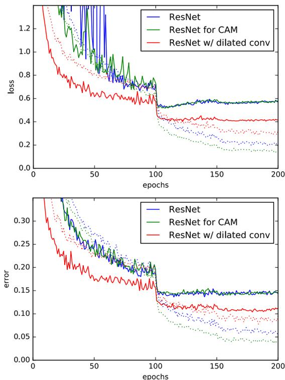
Figure 2. Loss(top) and top-1 error(bottom) curves of 3 CNNs in ImageNet50 classification. Training curves is drawn with dotted lines and validation curves solid lines.
