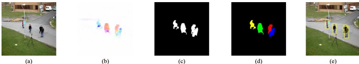
Figure 4. The whole procedure of our algorithm. (a) The raw frame. (b) Dense optical flow estimation. (c) High optical flow region extraction. (d) Motion segmentation by clustering. (e) The final results
