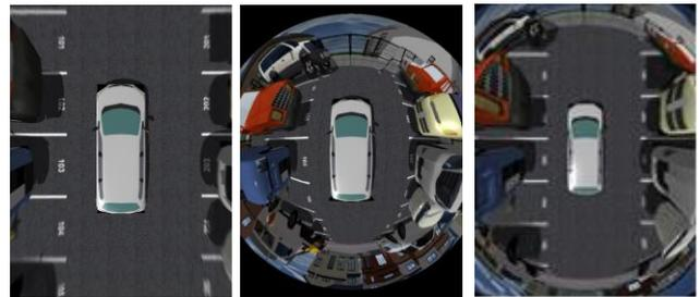
(b) Perspective projection on a plane (c) Equidistant projection on a half ball (d) Composite projection on a half pipe (proposed)
