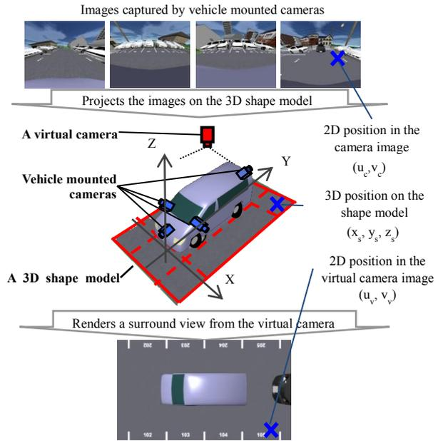
Figure 2. Process of generating a surround view.
