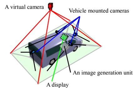
(a) A typical configuration of vehicle camera systems
