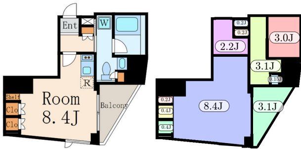
Figure 4: Room size estimation example: room sizes read with OCR in the input image (left) are propagated to unlabeled rooms (right).
