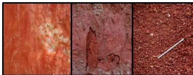
Figure 1. The Same mudstone in different disintegration states a) Low b) medium c) high.
