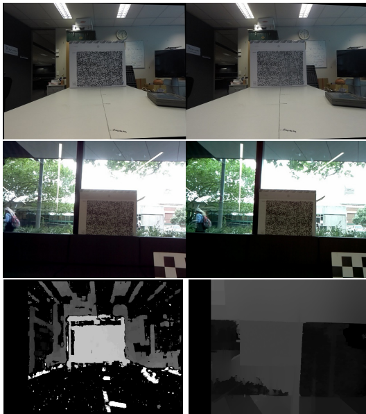
Figure 4: The RPi processing pipeline. From top to bottom: Indoor and outdoor rectified stereo pairs; corresponding disparity maps
