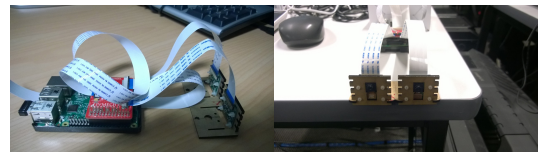
Figure 1: The Raspberry Pi with IVPort mounted, and camera modules attached
