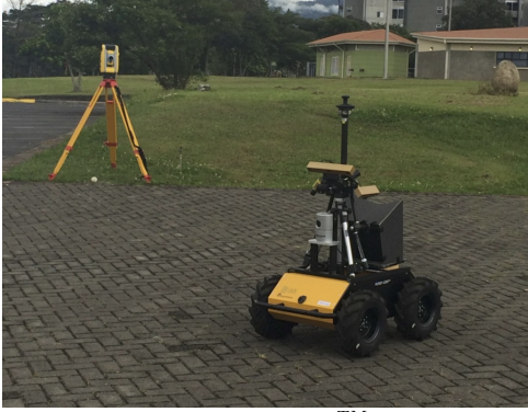
Figure 1. Clearpath Robotics TM Husky A200 TM rover platform and Trimble ® S3 robotic total station used for experimental validation.
