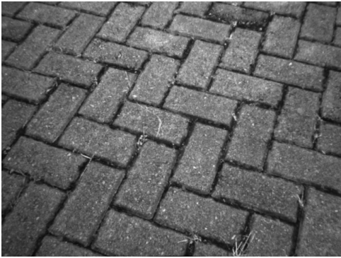
Figure 2. Example of an image with resolution 640 \times 480 \text{ pixel}^2 captured during experiment number 334. The camera is located at 77 cm above the ground looking to the left side of the rover tilted downwards 37 degrees.
