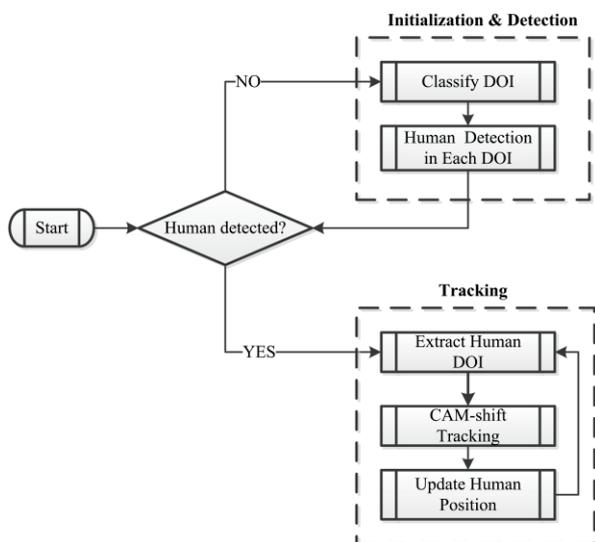
Figure 3. Human Detection and Tracking Model
