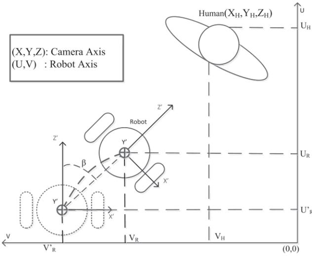
Figure 4. Human position under robot axis and camera axis
