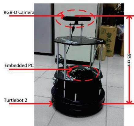
Figure 1. The mobile robot's hardware system
