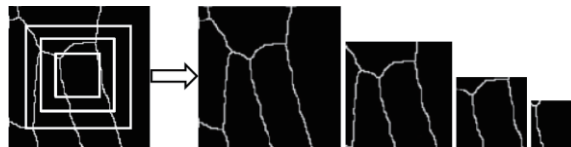
Figure 2. Inward partitioning of thinned image resulting in four sub-images of various dimensions ( 128 \times 128 , 96 \times 96 , 64 \times 64 , and 32 \times 32 pixels)
