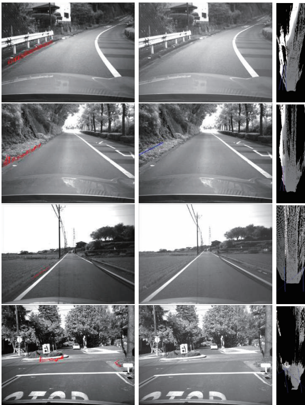
Figure 6. Detection results of proposed method (left) and DEM method (center/right). Road boundaries are curbs, vegetation, ditches and roundabout centers. (Best viewed in color)
