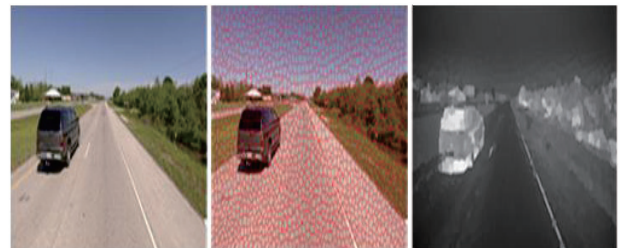
Figure 2. The saliency detection process. An input image (left) is over segmented to form a set of superpixels (middle). The saliency of each superpixel is determined to form a saliency map (right), in which the brighter the pixel the higher the saliency value is.
