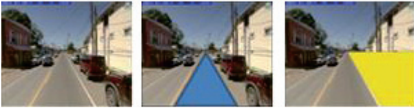
Figure 3. Road estimation and scene region extraction. In an input image ( left ), the traveling lane ( center ) can be identified to find the vanishing point, from which the road side image region can be estimated ( right ).
